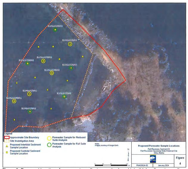
Figure 3: Proposed locations for porewater collectors and sub and intertidal sediment sampling
